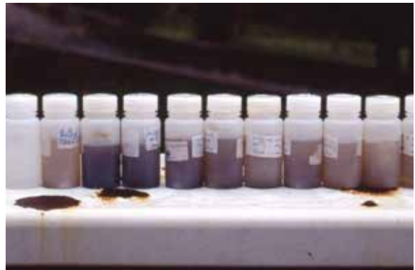
Figure 17.21. Water samples taken from a subsurface drain line when heavy rainfall followed liquid manure application. From left, water samples represent 15-minute sampling intervals from the onset of drain discharge. Photo by Larry Geohring.
