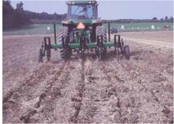
Figure 15.5. Left: Subsoiler shank provides deep compaction relief (wings at the tip provide lateral shattering). Right: Zone building provides compaction relief and better rooting with minimal surface disturbance. Right photo by George Abawi.
