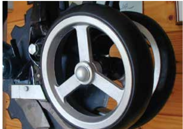
Figure 16.6. Left: A no-till seed drill requires no tillage or seedbed preparation for narrow-seeded crops or cover crops. Right: The cross-slot opener used in no-tillage planters. The disk slices soil, the inverted T blade allows seed and fertilizer placement on opposite ends of disk, and the packer wheels (right side) close and firm the seedbed.
